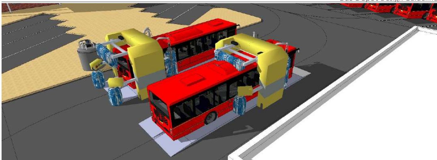
Figure 44: View of washing area showing gantry washers
