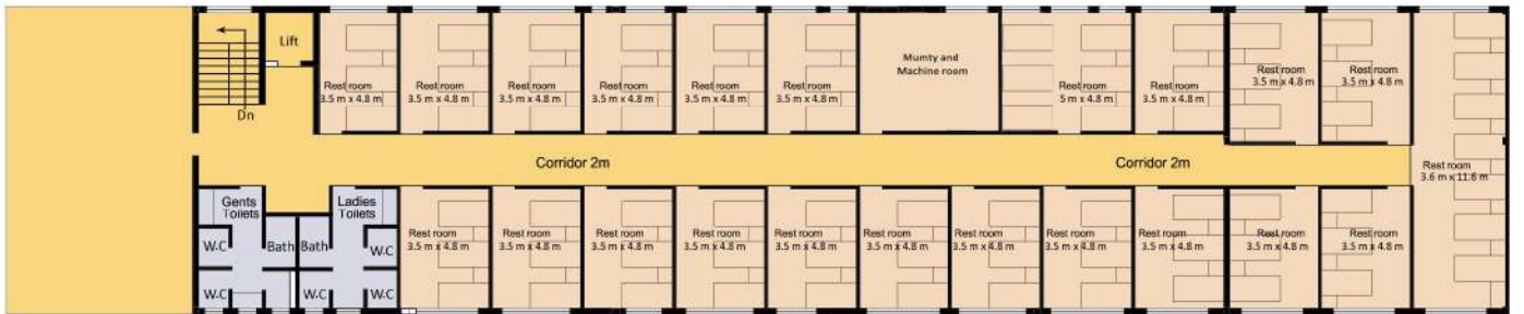
Figure 53: Administration block second floor plan
