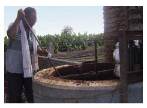
Vijay Ingle stirs the slurry in the biogas digester tank
