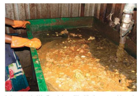
The slurry waste from a plant's digester is rich in nutrients and can be used as fertiliser
