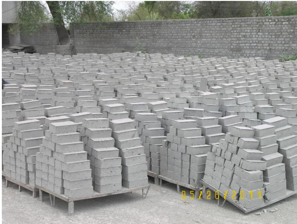
Figure 5: FaL-G blocks stacked for curing
