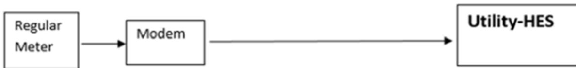
Figure 4-3: Automated Meter Reading Architecture
