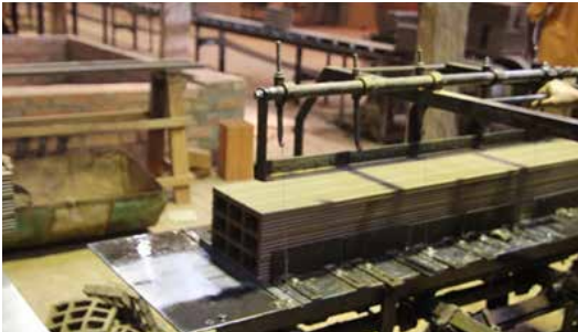
Mechanised hollow clay block manufacturing
