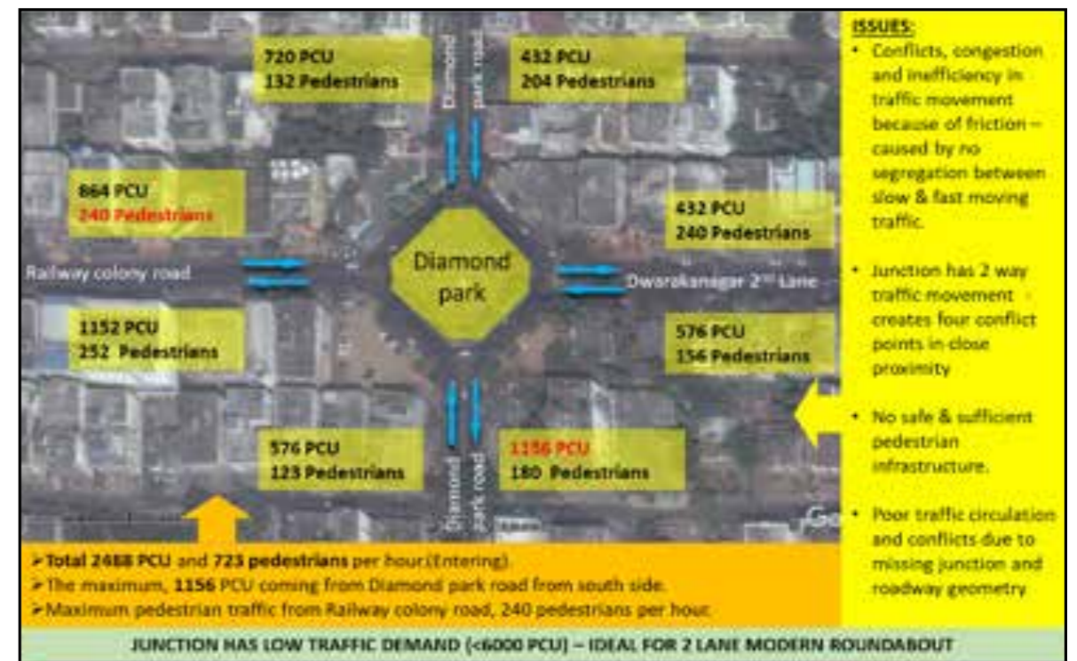
Figure 11: Existing peak hour Arm-wise Traffic (in PCU) and Pedestrian Count
