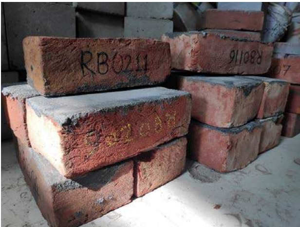
Figure-A2.16: Photograph of mortar filled bricks ready to be tested.
