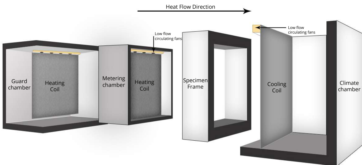
Figure 2: Exploded view of the Guarded Hot-Box apparatus
