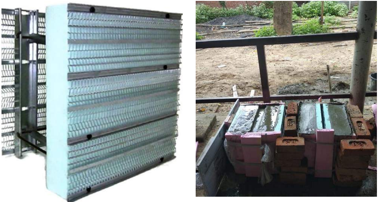
Figure 28: Photograph of an insulated coffer panel sample without concreting (left), Photograph of concrete poured in-situ in the insulated coffer panel sample (right). Source: (left) (BMTPC, 2018c)
