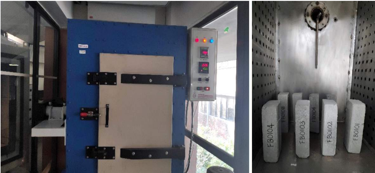
Figure-A2.4: Photograph of the Inert Gas Oven (left) & bricks prepared for drying (right)
