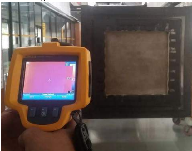
Figure 7: Photographs showing thermal imaging (left) and testing of Rat trap bond wall assembly in GHB
