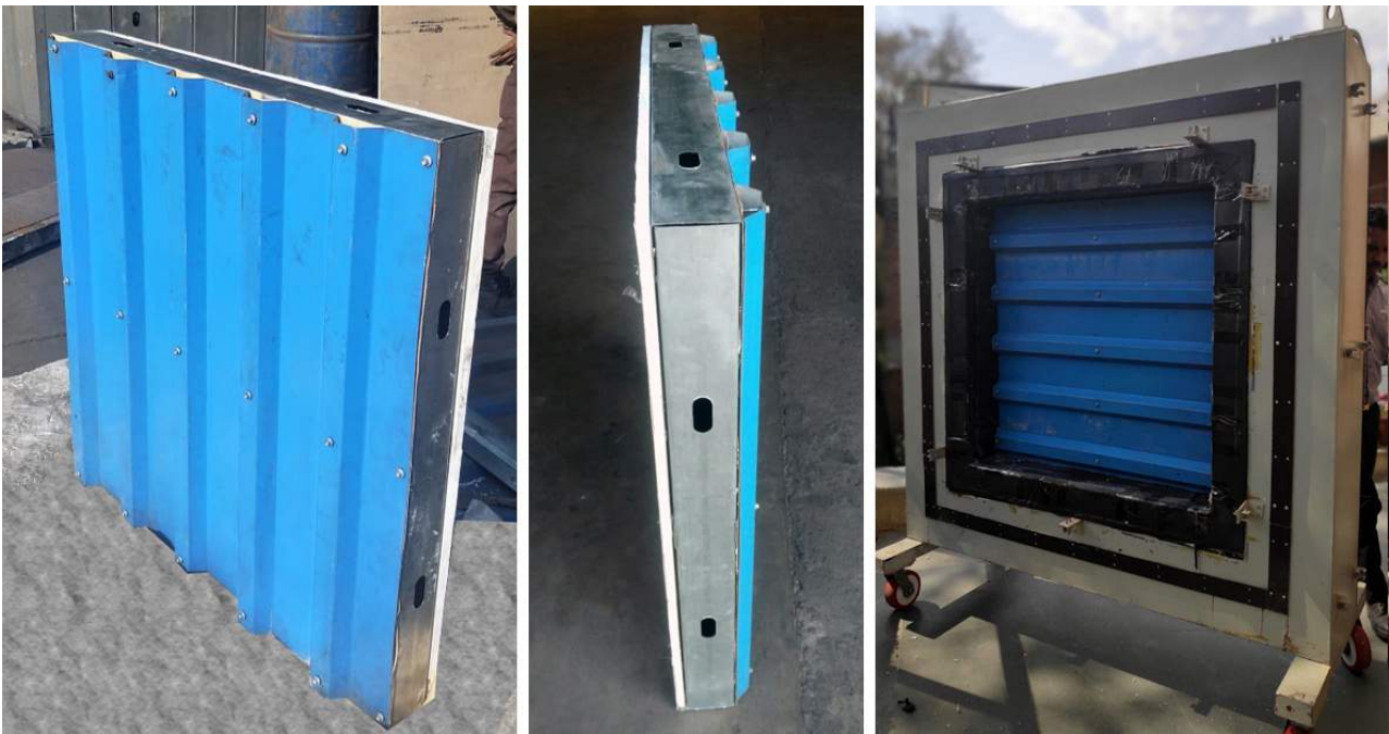
Figure 17: Photograph of LGFSS with PPGL sheet wall sample (left) & the sample installed within specimen frame of GHB (right)
