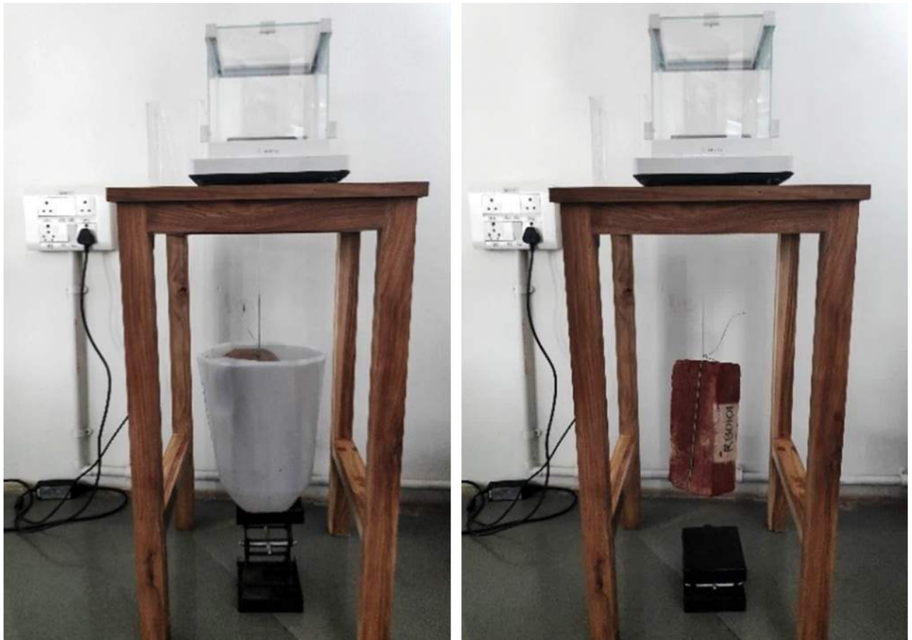
Figure-A2.14: Photograph showing measurement of suspended weight (S)(left) and saturated weight (W)(right) as per the procedure.
