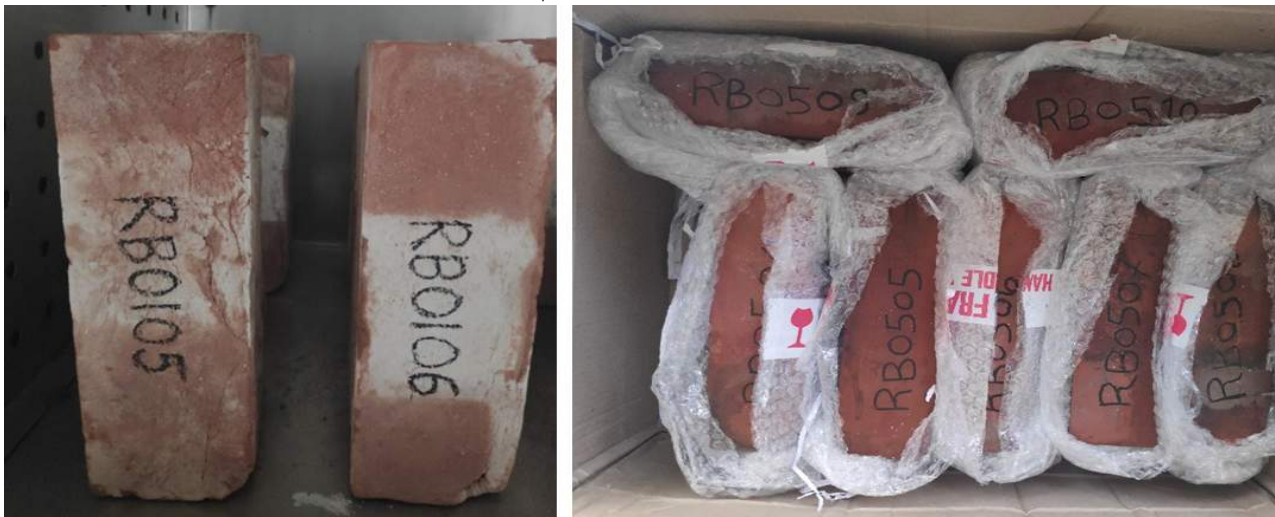
Figure-A2.1: Illustration to explain sample tag (top) and photograph of tagged bricks belonging to set 01 (left) & set 05 (right)
