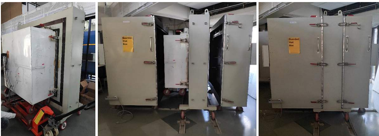
Figure 3: Photographs of the metering chamber attached to the specimen frame and the entire assembly of GHB opened up and closed.
