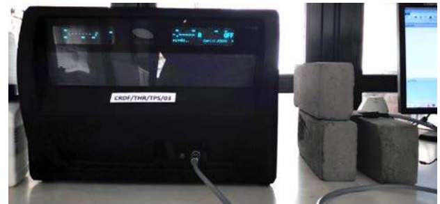
Figure-A2.2: Photograph of thermal constant analyser testing brick samples using transient plane source method
