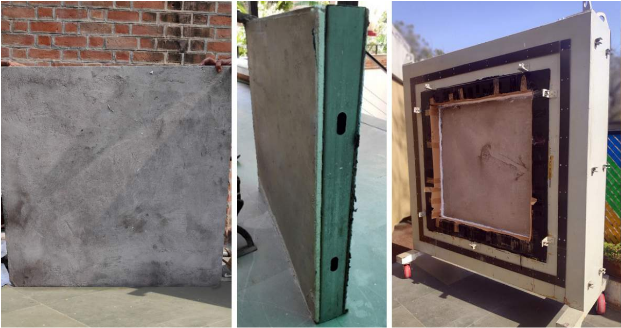
Figure 16: Photograph of LGFSS with EPS wall sample (left) & the sample wall installed within Specimen frame of GHB (right).
