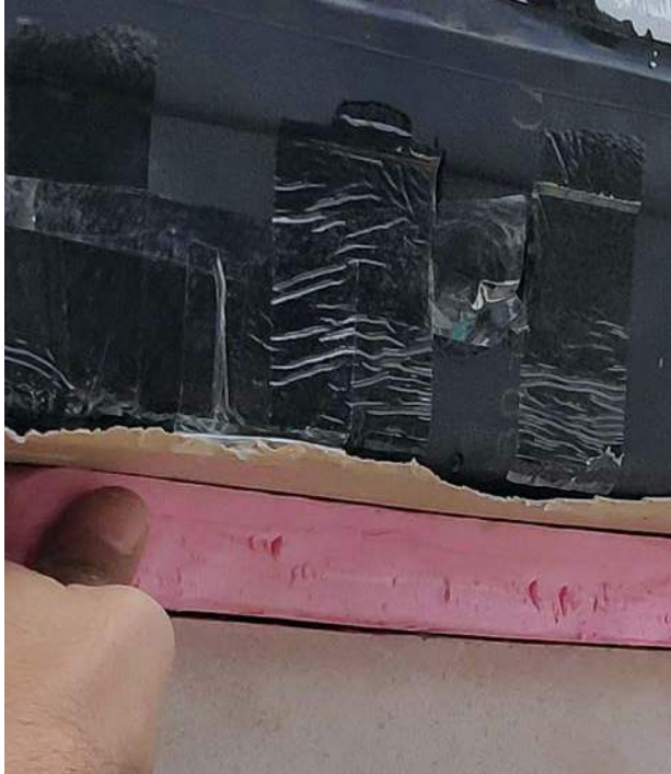
Figure 8: Photographs showing sealing procedure with XPS (left) and silicone sealant (right) to avoid heat transfer through gaps
