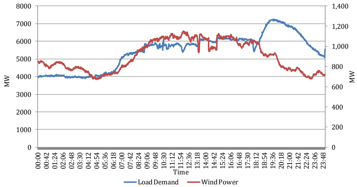
Figure 5.9: Variation in wind power output and load demand on 1 Aug'11
