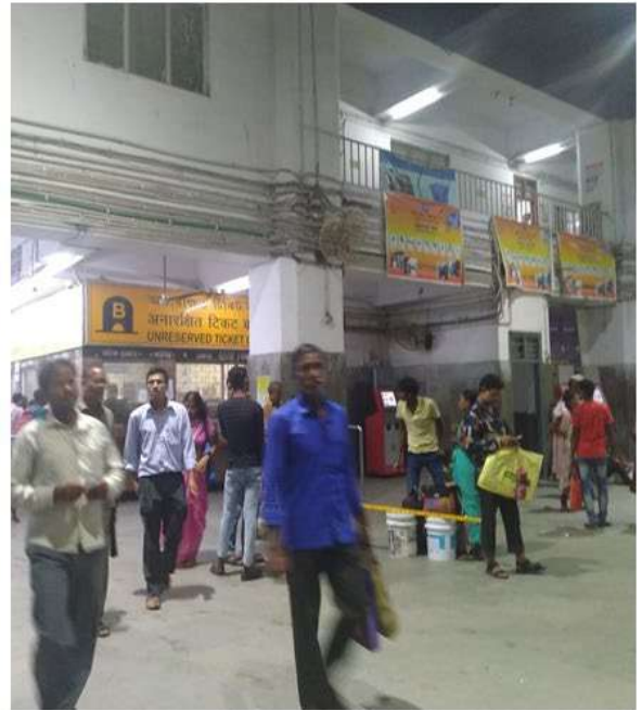
Figure 30: Ad hoc addition of wires, without accounting for load and impact on structure -- Sealdah Railway Station
