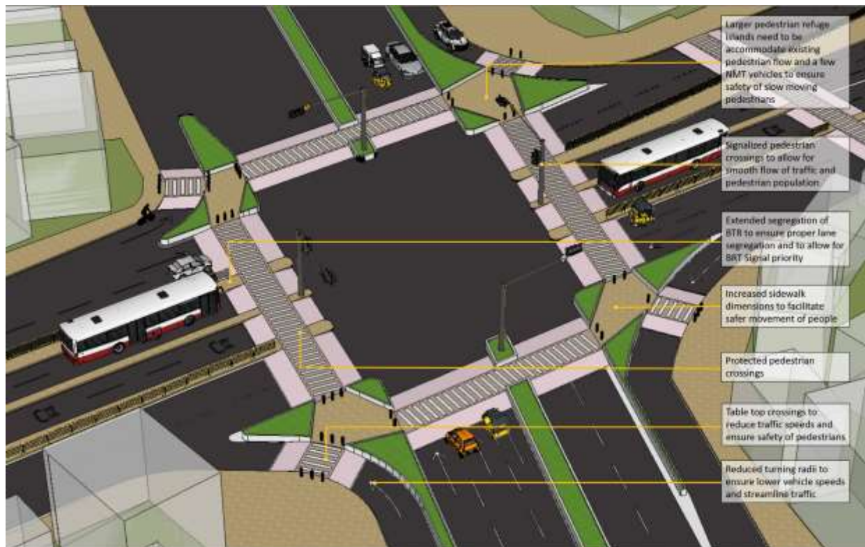
Figure 10: Improved junction design at NAD junction
