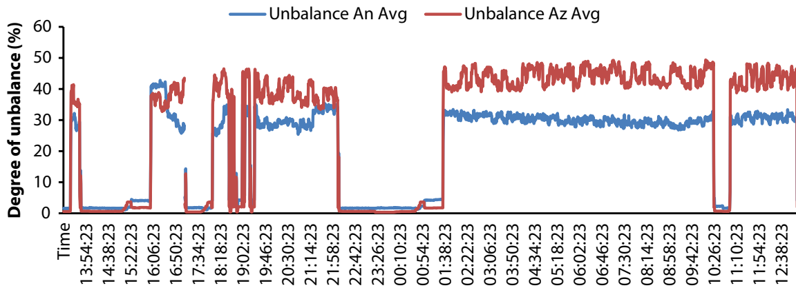
Figure 33: Variation in degree of current unbalance with reference to negative and zero sequence for Kasba depot measurements
