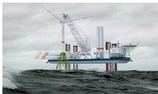
Figure A13.1: Wartsila high performance turbine installation vessel
