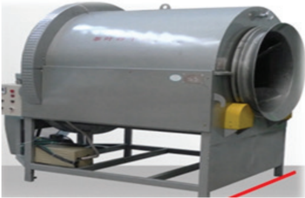
Figure 3. Withering fan with electric heating assembly
