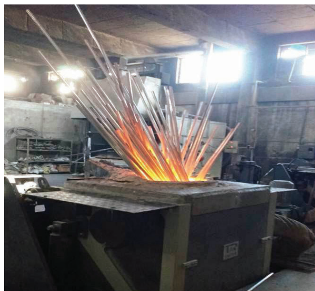
Energy inefficient operating practice: large sized raw materials charged into induction furnaces
