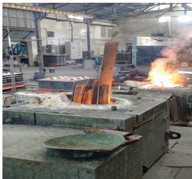
Energy inefficient operating practice: large sized raw materials charged into induction furnaces
