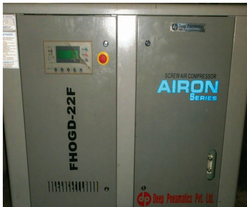
Replacing reciprocating air compressor (L) with VFD-based screw air compressor (R)
