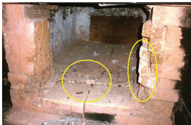
Relining shell baking furnace: (L) damaged lining; (R) repaired lining
