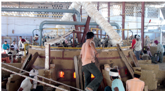
Auxiliary furnace in glass bangle production – Firozabad cluster
