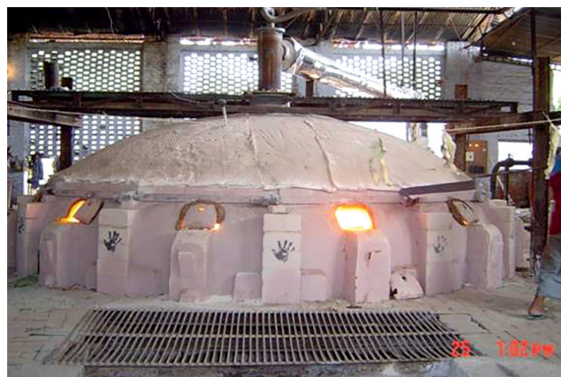
TERI-design recuperative pot furnace for glass melting
