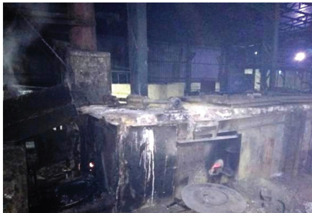
Lead bath used in wire drawing
