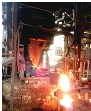
Coke-fired cupola melting furnace
