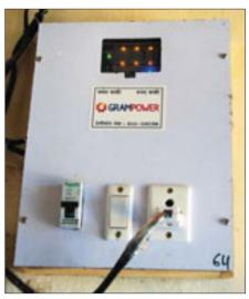
Gram Power, a micro-grid technology provider, has installed pre-paid smart meters in Pali district of Rajasthan
