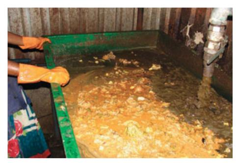
The slurry waste from a plant's digester is rich in nutrients and can be used as fertiliser
