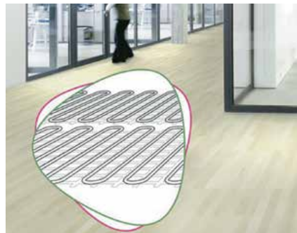
Figure 10: Radiant floor cooling system layout (Rehau.com, 2017)
