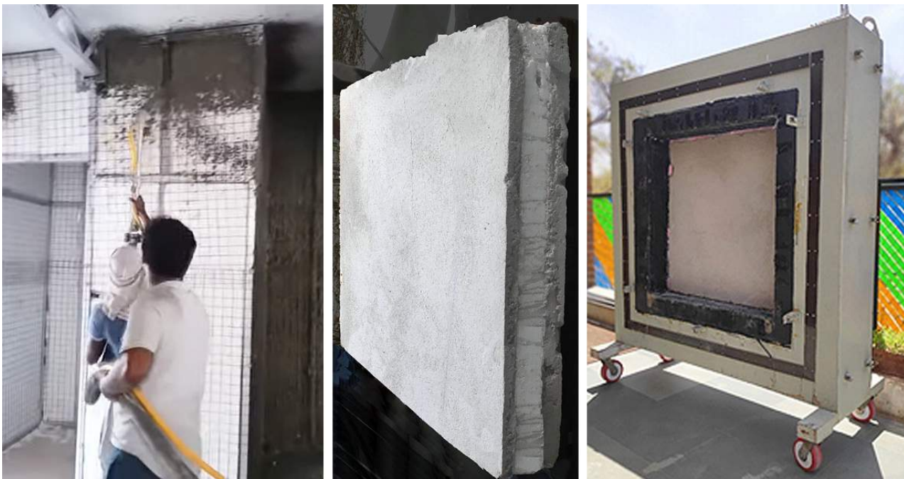
Figure 20: Example of on-site shotcreting (left), Sample of EPS core panel received from the manufacturer (middle) and EPS core panel fixed into the specimen frame of GHB(right) Source: (left) (BMTPC, 2018a)
