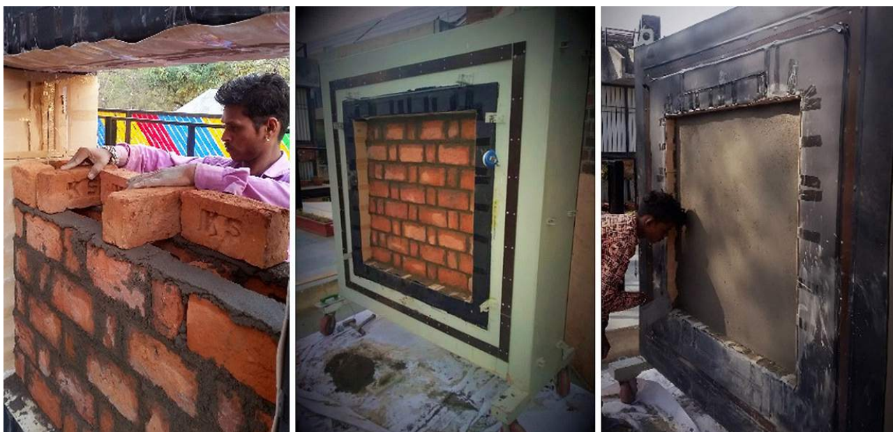
Figure 12: Photograph showing the construction of Rat trap bond wall within the specimen frame of GHB.
