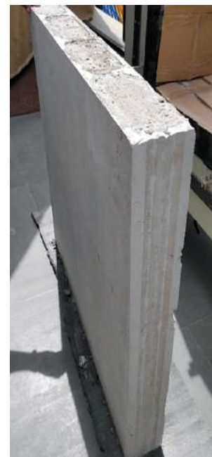
Figure 23: 3D illustrations (left) and photographs of the GFRG Panel samples: unfilled, partly filled and fully filled (right)
