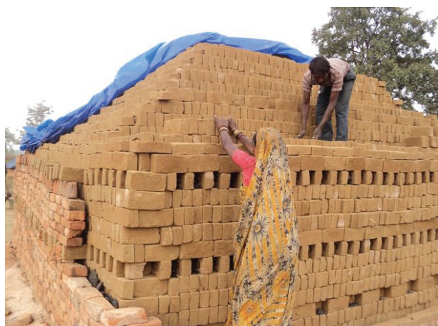
Arrangement of bricks in a clamp
