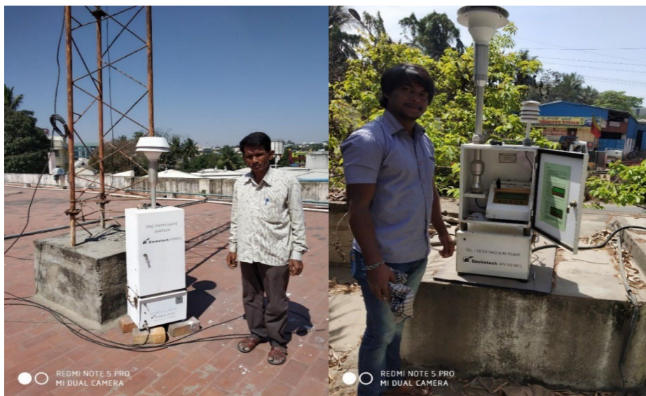
Figure 2: Fine particulate sampler (Envirotech APM 550 MFC) used for PM 2.5 sampling
