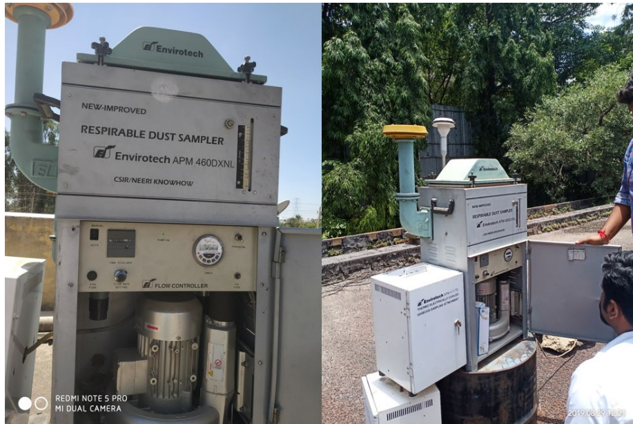
Figure 1: Respirable dust sampler (Envirotech APM 460DXNL) used for PM 10 sampling
