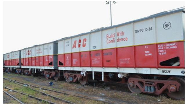
**Figure 15:** BCCW wagons for bulk transport of Cement/Fly Ash
