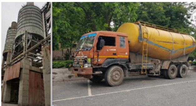
**Figure 2:** Photograph showing Fly Ash Loading Silos and Road Bulklers
