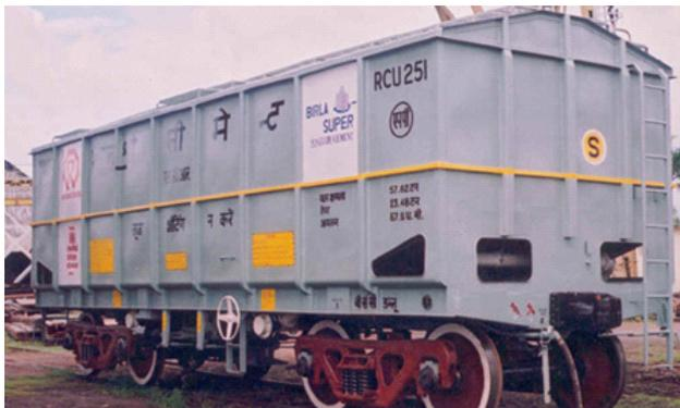
**Figure 14:** Covered Car "BCCW" wagon for bulk transport of Cement/Fly Ash
