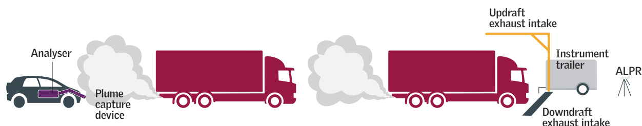
Figure 2: Types of extractive systems (right: exhaust plume chaser; left: stationary air sampler)
