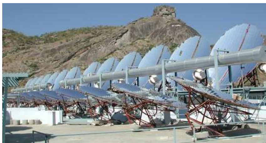
Figure 63 Parabolic concentrating solar cooker
