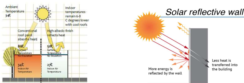
Figure 2 Representation of solar radiation 1 and effect of SRI coating
