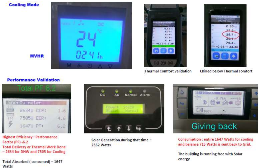
Figure 24 e-Manager for auto switching between Grid and Renewable
